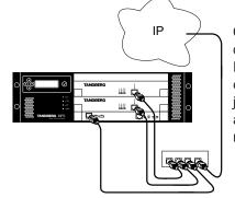
Connect a LAN cable from the Ethernet socket of the board just installed and to your network.
